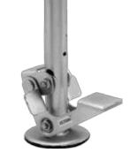
Designed to hold portable equipment in a desired location. Intended for use on level surfaces. Floor lock is activated by toe pressure on the extension pedal or released by toe touching one of the dual retractable plates. The large non-skid brake pad, under high spring compression, holds the portable piece of equipment until released. For best results, units should be used in pairs.
