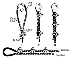
NOTE: Mechanical spliced or flemished eyes slings are the preferred method of wire rope sling construction.
