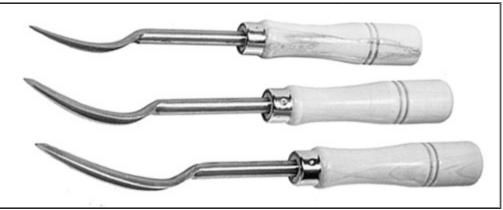
The perfect bearing scaper. Absolutely non-chattering. Manufactured with the utmost care from the highest grade tool steel. Each scraper is deeply grooved and hollow ground and carefully tempered. Hardwood Handle. Blade polished.
