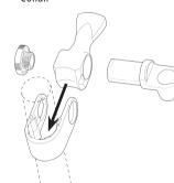
Screw Threaded Cap onto end of Hand Shower Holder. A coin may be used to assist in tightening Cap; however, be careful not to over tighten.
