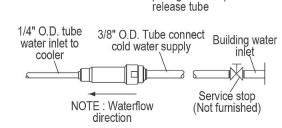
These products are designed to operate on 20 psi to 105 psi supply line pressure.
