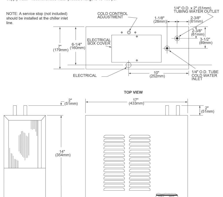
NOTE: It is important to insure proper ventilation. If this remote chiller is physically placed against barrier or in enclosure of any kind, 4" (102mm) air space must be allowed on all sides.
