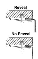
Mounting bracket assembly provides a secure installation.
