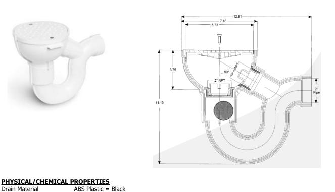
Grate Material Grate Open Area Grate Load ABS Plastic = Black PVC Plastic = White Polypropylene (black or white) 7.25 in.<sup>2</sup> Light\*
