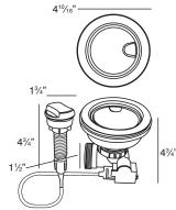
Turn the remote knob to open and close drain. Water drains easily when cover is in place. Cover flips up with easy touch.
