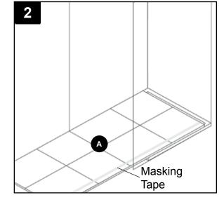
3. If needed, place 1/16 in. thick shims (not included) at the base of the back panel's (A) installation site. Trial fit the back panel (A) on the shims and use a sanding block if any fine adjustments are needed. Remove back panel (A) from wall and clean the back of the panel (A), the wall board and any other area that will be in contact with the silicone (K) with denatured alcohol and a clean rag (both not included).
