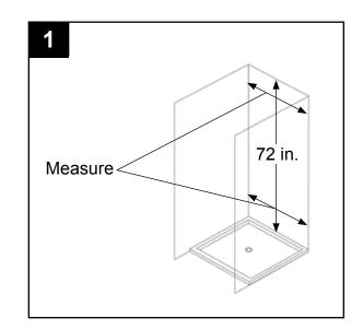
Check the measurements, and then place masking tape (not included) over the area where the saw (not included) will contact the finished side of the back panel (A). Cut the back panel (A), and make any final adjustments to the cuts with a sanding block (not included).
