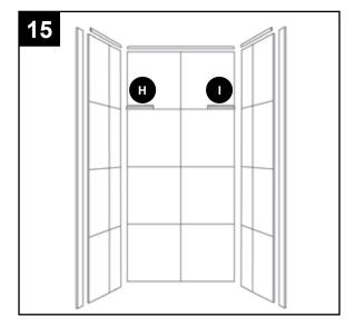
Once installation is complete, seal all the joints with silicone adhesive/sealant (K). Note: Clean all joints with denatured alcohol before applying a uniform bead of silicone adhesive to the joints.
